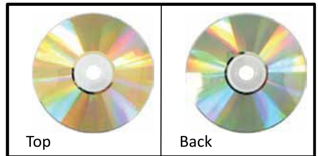
Aging Test: Gold Archival CD-R vs Std CD-R at 80C/80% RH
